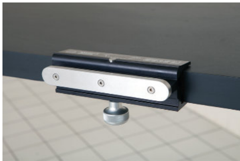
Clamp-on Accessory Rail For attaching accessories to table top. Rail is 6" (15,2 cm) long x 3/4" (95 mm) thick x 1-1/8" (3 cm) high.
